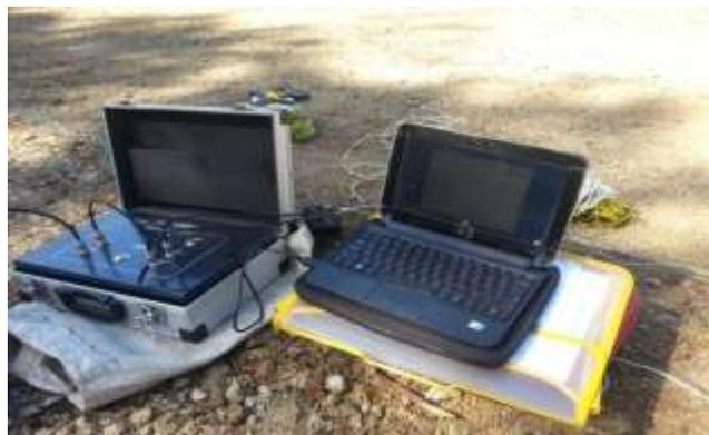
**Gambar 3. Multi Channel Resistivity merk S-Field**
