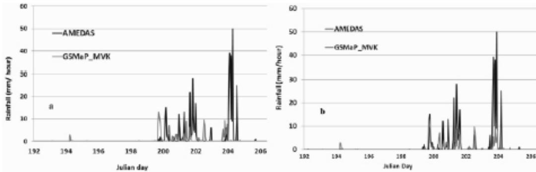
Figure 5 Rainfall pattern before the flood occurred in Asotohime city, 12 July 2012 (a); and after time lag matching (b).
