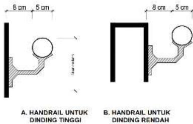
Gambar 12 Detail Handrail
