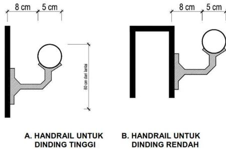
Gambar 12 Detail Handrail
