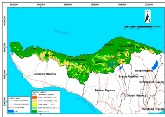
Figure 3. Hazard map of landslides using Soil Stability Index Mapping (SINMAP).
