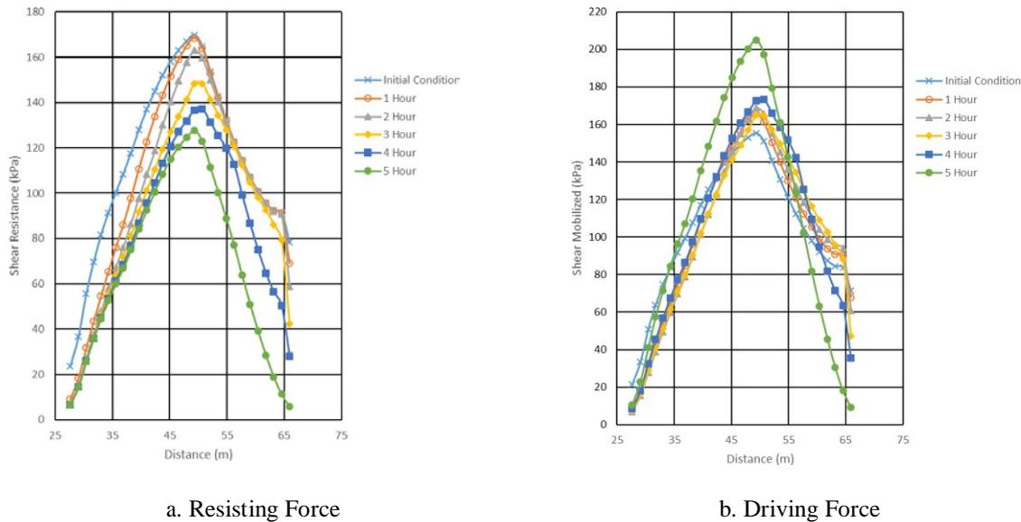
**Figure 7.** Resisting force and driving force at the sliding surface
