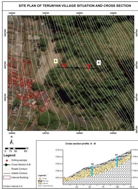
a. Cross section A-B and Drilling sample
